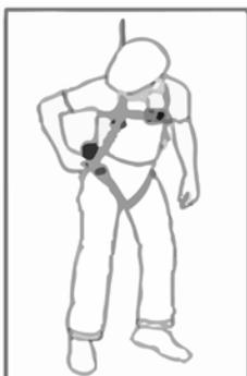
1. Un-zip the pouches fitted on both sides of the Harness.
